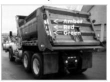
So, unlike flashing green traffic signals (extra credit: what do those mean?), flashing green vehicle lights tell you to exercise caution around snow and ice removal equipment. Be nice, they're trying to make the road safer for you.
